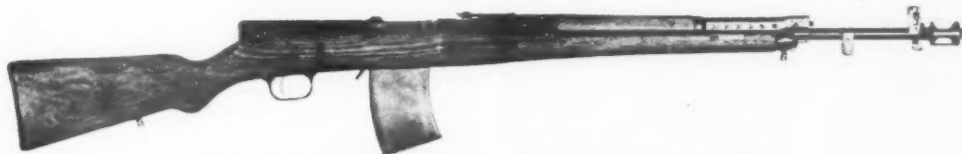
Simonov 7.62 mm. rifle was Russia's first semiautomatic. Reportedly capable of fully automatic fire, the rifle is fed from a 15-round magazine
